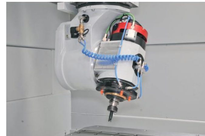
5 axes milling unit with direct drive technology
