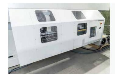
Dust and chips management with integrated conveyor, new telescopic hood with high efficiency fluidynamics
