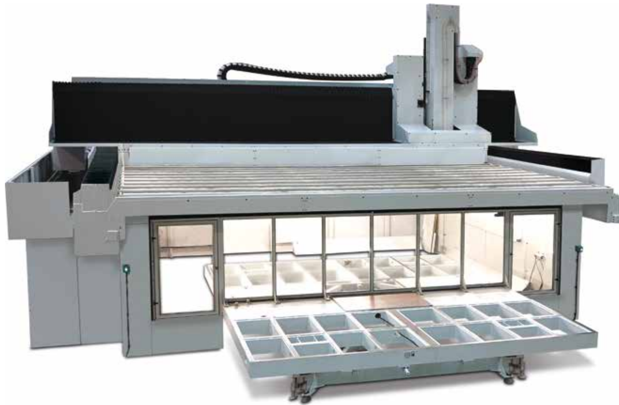
ROTARY TABLE: SIMPLIFIES LOADING/UNLOADING OUTSIDE THE MACHINE AND ALLOWS PENDULUM CYCLE USING THE COMPLETE WORKING AREA
