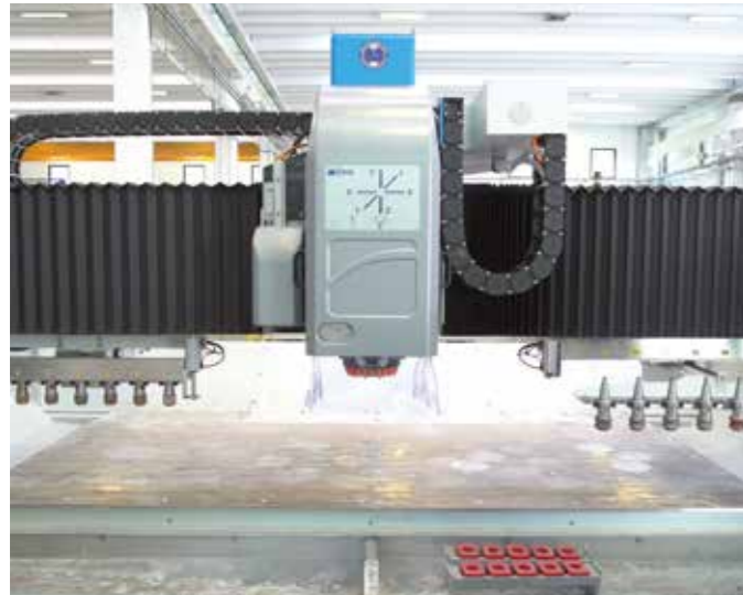
UNDERBEAM MAGAZINE: 8-station tool magazine housed below the machine beam, usable for grinding wheels, scabble wheels, core drills, inscription and engraving tools for natural stone, composite, and ceramic slabs.
